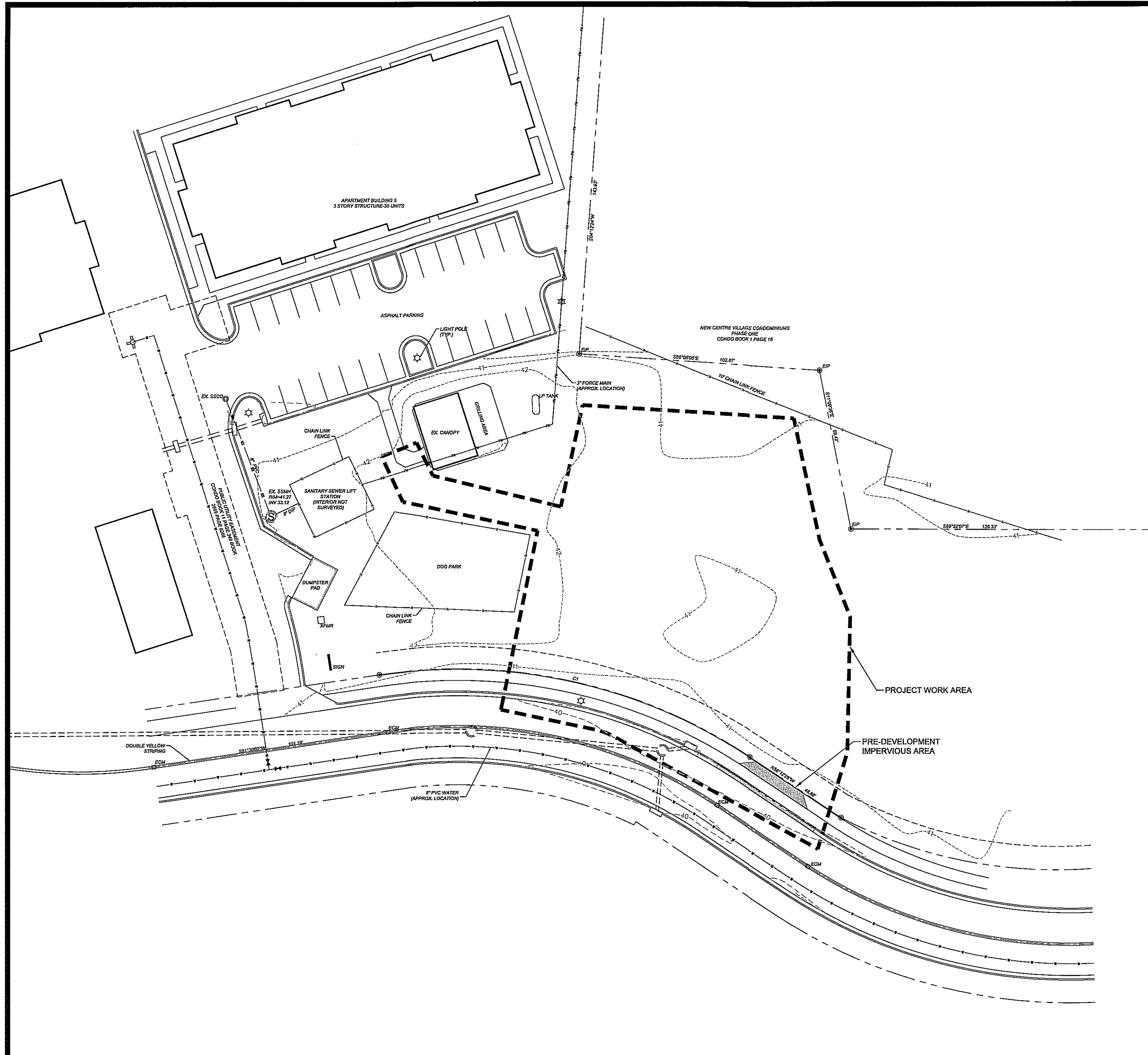
PRE-DEVELOPMENT DRAINAGE AREA AND IMPERVIOUS AREAS SCALE: 1"=30'
